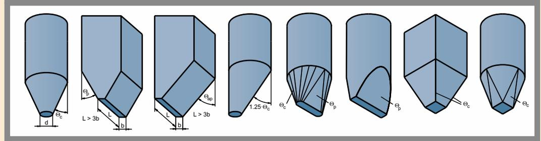
Hopper wall slope in dependence on local hopper diameter
