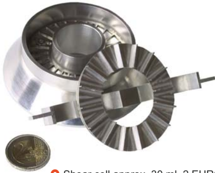
Shear cell approx. 30 ml, 2 EURO coin
