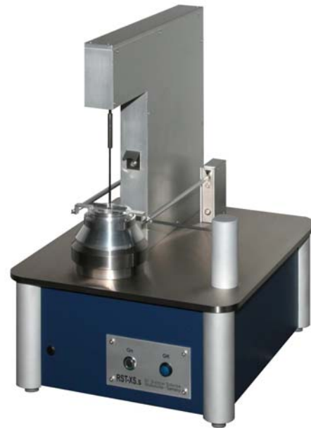
● Ring shear tester RST-XS.s
